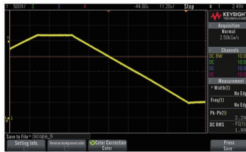
▲ CC to CV/CC to CC Transition Waveform
